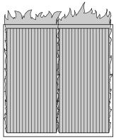
Figure 19 - Incorrect Burner Flame Pattern (Model VN12 Shown)
